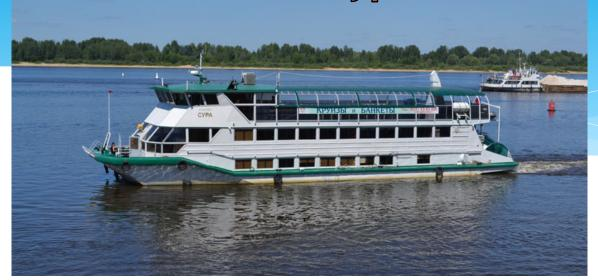
Invention triggered by physical navigational conditions: winged propeller gave ability to operate this vessel on small rivers even without quays, piers or berths but directly "landing" it on the river shore banks ("bow into shore" action). Self ungrounding capacity provides either the commercial advantages.
