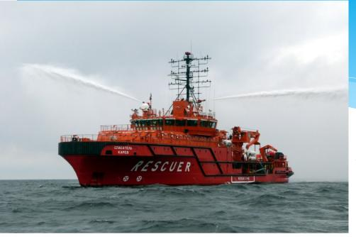
Ice-breaking + Rescue vessel MPSV 07 type
