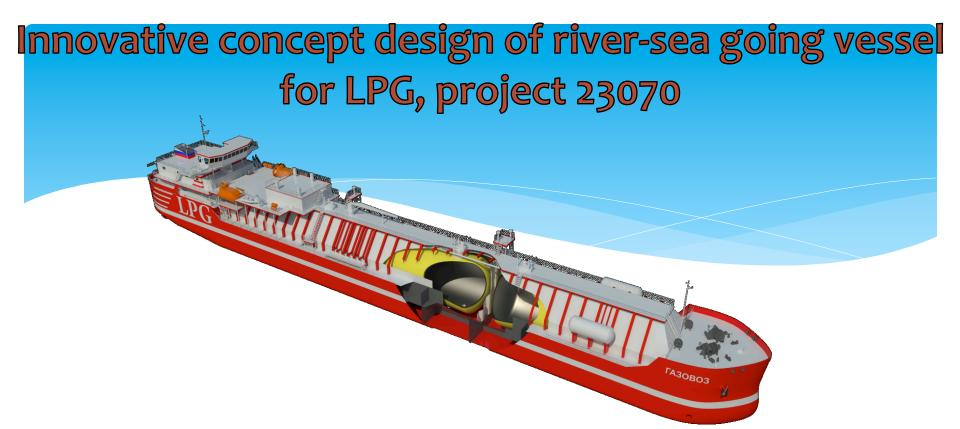
Length<sub>max</sub> x breadth<sub>max</sub> x midship depth: 140.2 x 16.6 x 6.7 m;
